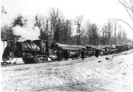
The Lombard steam log hauler was the original crawler type overland tractor. It had crawler treads and skids in front for steering. It required 4 men (and engineer, fireman, pilot or steersman, and conductor) to operate it.
